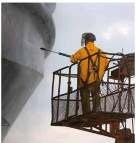
It is recommended that, in line with industry regulations, all WATERBLAST assemblies are pressure tested to 1.5 times the maximum working pressure.
